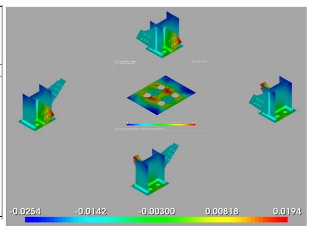
Welds are modelled with a number of equally-spaced linear elements, glued to the mid-surface of the welded plates by rigid offsets. For each weld element the internal forces axial, parallel and perpendicular shears are obtained. AISC provides close check formulae for the welds using the integration of these forces, which can be immediately computed for each loading combination and for each weld, so the checks are immediate.
