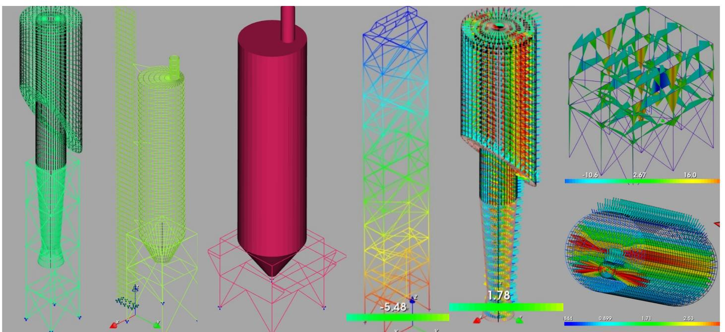
The analysis of the connection by means of finite elements does not rely on any basic assumption regarding the behaviour of the connector subcomponents. All the components were modelled in exact spatial positions, taking into account the parameters that define the stiffness of each of them (length, diameter and number of bolts, length of welds, throat section, . . . ). That way, the model does not neglect any part of the response, all the forces flow correctly between components.
