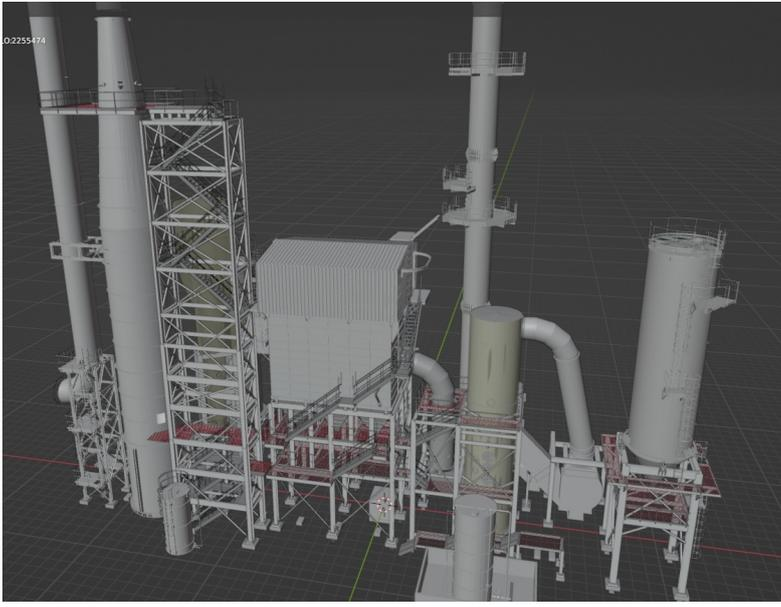
The Veolia Value Park (VVP) plant is located in Jubail Industrial City, Kingdom of Saudi Arabia, and consists of an Integrated Waste To Energy (IWTE) Central Utilities and Valorization Plant that will precondition liquid and solid hazardous industrial waste (Class I and Class II), burning it and recovering energy in the form of steam for use within several industrial applications.
