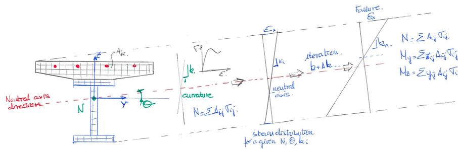
Figure 3. Generic process to obtain one point of the interaction diagram
