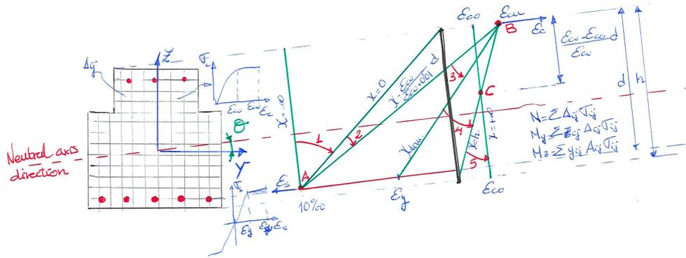
Figure 2. Process to obtain a set of points of the interaction diagram for a RC section
