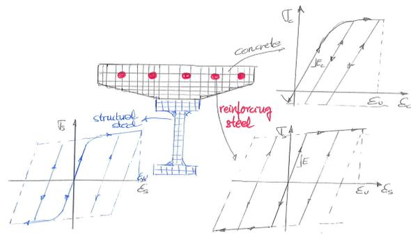
**Figure 1.** Fiber model of a cross section made up of various materials
