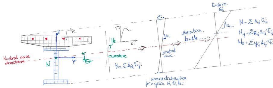
Figure 3. Generic process to obtain one point of the interaction diagram
