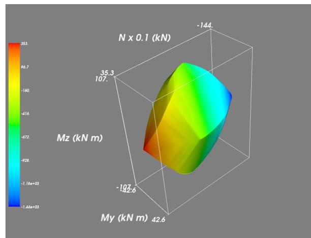
Figure 5. Example of interaction diagram generated by XC
