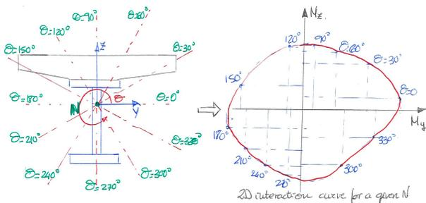
Figure 4. Process to obtain a failure curve for a certain value of the axial load
